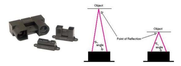
If the IR signal is detected, it is safe to assume that an object is present
