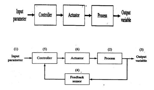
An **open-loop control** system utilizes a controller or control actuator to obtain the **desired response**, as shown in Figure. The open-loop control system utilizes an actuating device to control the process directly without using device. An example of an open-loop control system is an **electric toaster**.
